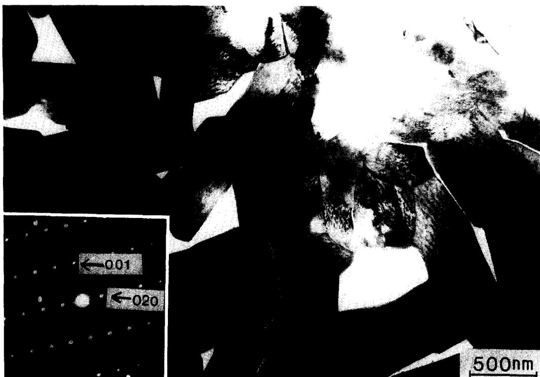
FIG. 6. TEM picture of MoO<sub>3</sub> crystallites (sample 2), including as an inset the electron microdiffraction pattern for the central crystallite (indicated by a white arrow).
